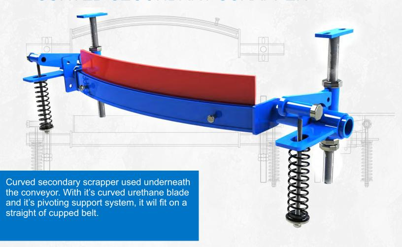
Secondary scrapper to clean fines left by a primary scrapper on straight or cupped belts. Usually installed underneath the conveyor outside the discharge chute.
