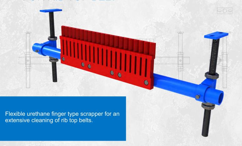
Finger type scrapper used to clean rib top belt up to 1/2" thick from sticky material. Usually installed behind drive pulley an ideally in the discharge chute.
