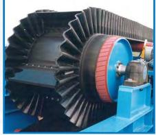
Sturdy construction using two sealed bearings mounted on 1 1/4" steel or stainless steel shaft. Optional threaded or extended shaft are available.
